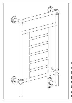
Liquid-filled models MUST be installed with the wire cover tube / junction box being positioned at the bottom.
