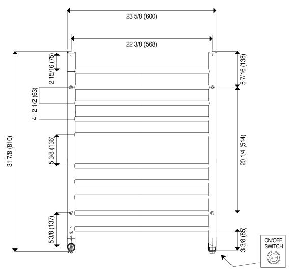
Note: Drawing shows back of unit. Power connection on the right when mounted on wall.
