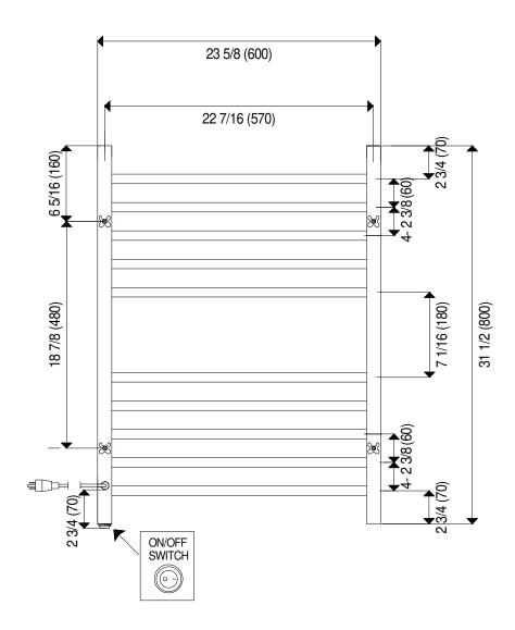
Note: Above drawing shows back of unit. Power connection on the right when mounted on wall.
