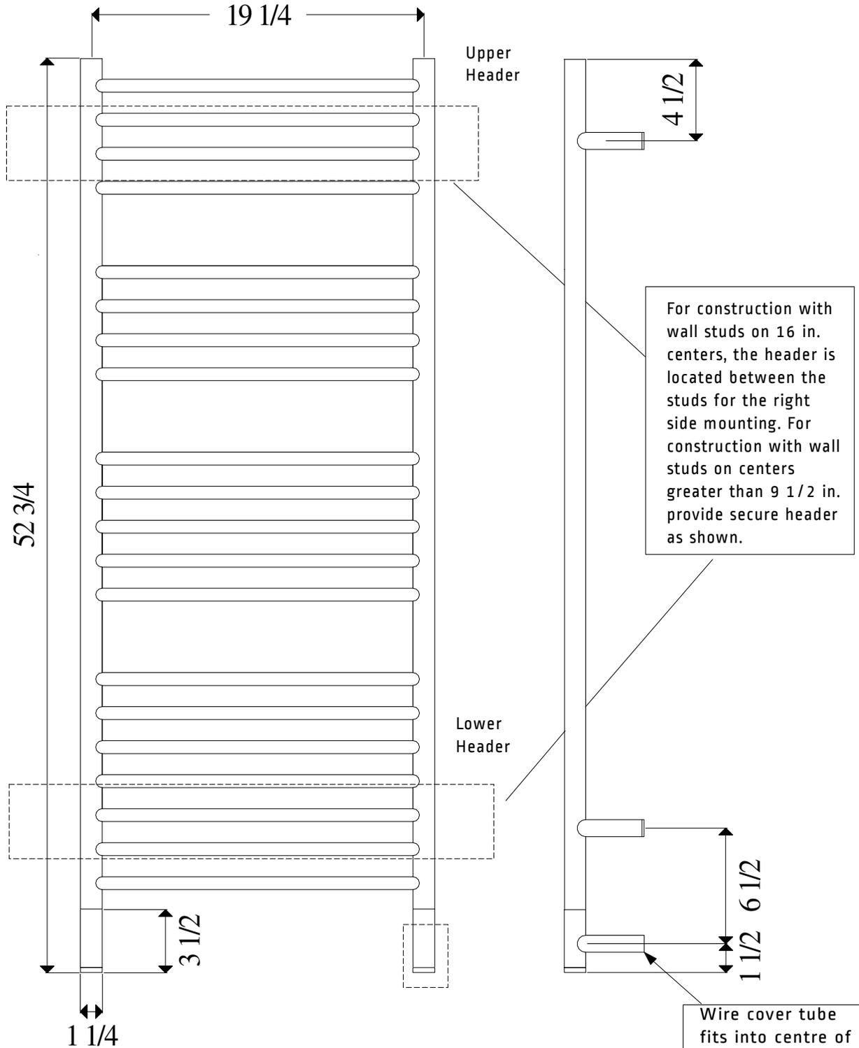
For construction with wall studs on 16 in. centers, the header is located between the studs for the right side mounting. For construction with wall studs on centers greater than 9 1/2 in. provide secure header as shown.
