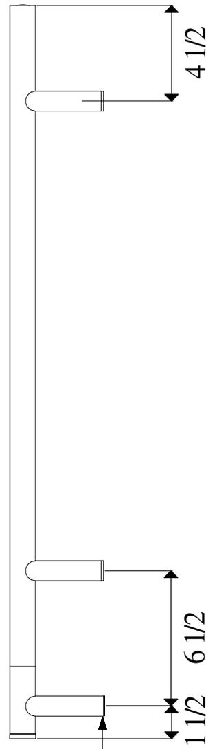
Wire cover tube fits into centre of cover plate which fits over single gang box
